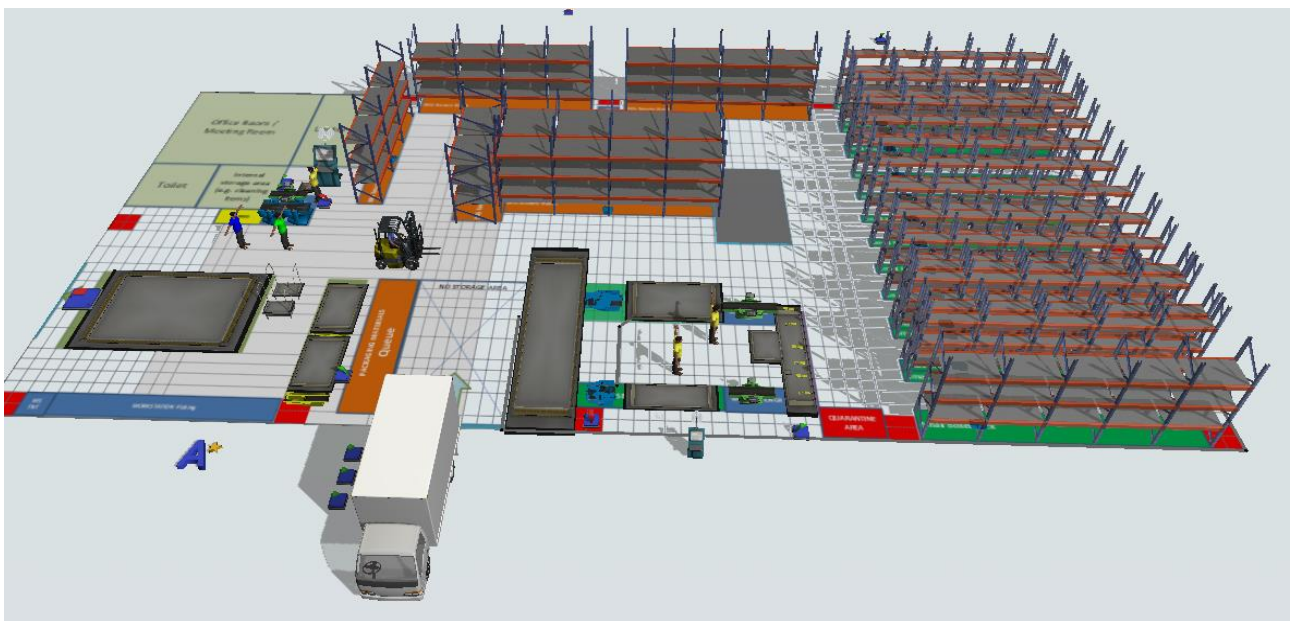
Fig. 7. Model of new situation of warehouse
