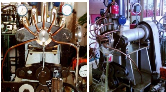
Fig. 1. Radial bearing during measurements
