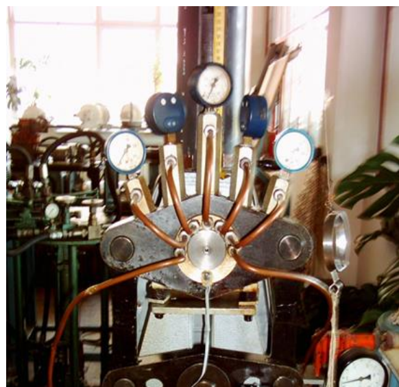
Fig. 1. The experimental stand with the ADXL 190 WQC acceleration sensor
