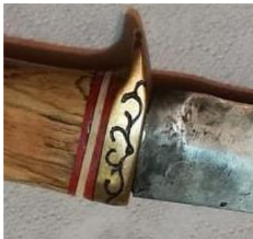
Fig. 1. Results of electrochemical engraving applied to a workpiece obtained by sintering granules of different alloy steels
