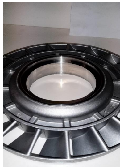
Fig. 2. Test workpiece before broaching of internal contoured surfaces
