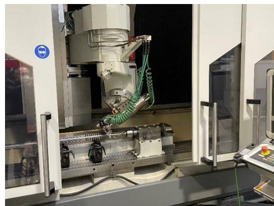
Fig. 6. Grinding of broaching tool on the sharpener
