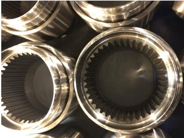
Fig. 3. Workpieces after broaching with a profile shape
