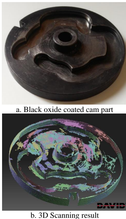
Fig. 5. Results of the 3D scanning operation of the black oxide coated part
