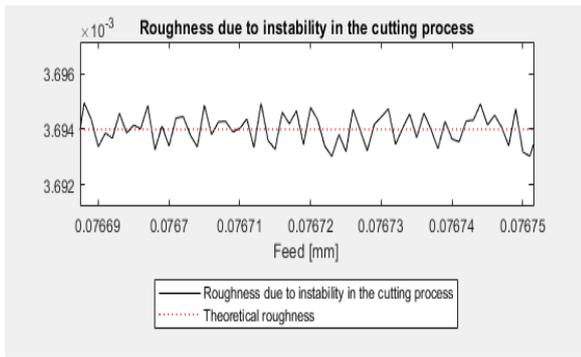
Fig. 4. Difference between theoretical surface roughness and surface roughness caused due to instability in the cutting process
