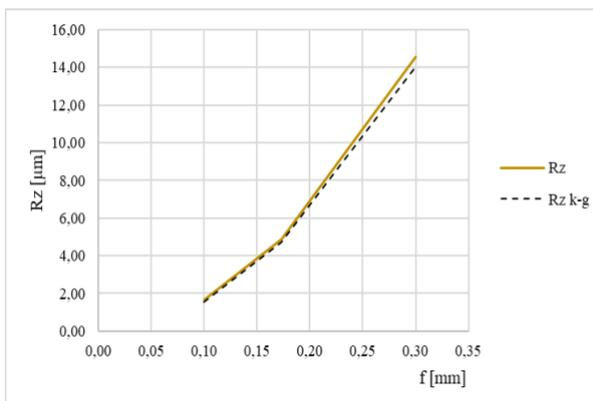
Fig. 7. Development of the surface roughness parameter  $R_z$  depending on the feed for the tool tip radius  $r_\epsilon = 0.8\text{ mm}$
