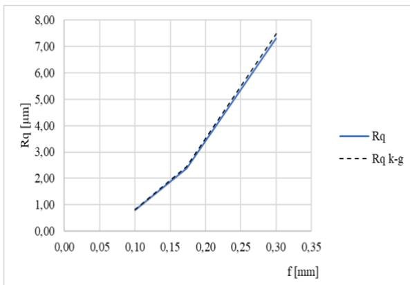
Fig. 6. Development of the surface roughness parameter  $R_q$  depending on the feed for the tool tip radius  $r_\epsilon = 0.4\text{ mm}$
