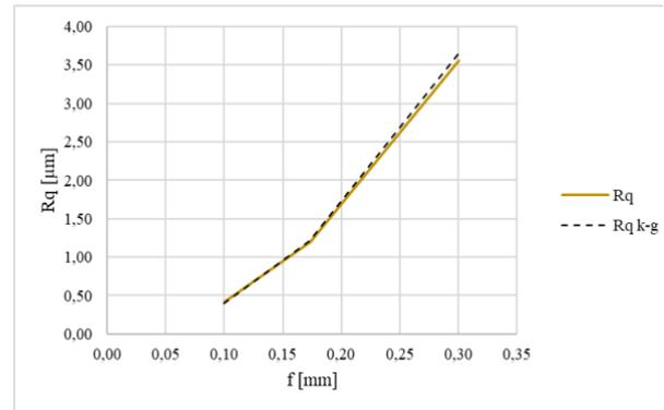
Fig. 8. Development of the surface roughness parameter  $R_q$  depending on the feed for the tool tip radius  $r_\epsilon = 0.8\text{ mm}$
