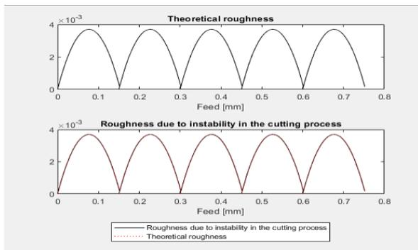
Fig. 3. Model of the theoretical roughness and the roughness caused due to instability in the cutting process
