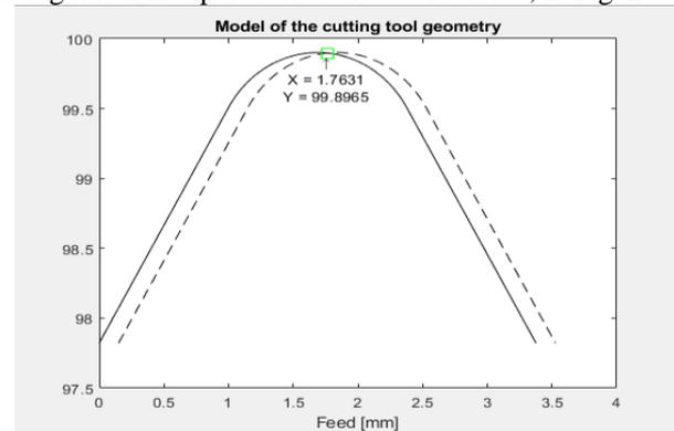
Fig. 2. The intersection between 2 toolpaths
