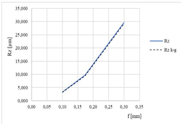
Fig. 5. Development of the surface roughness parameter  $R_z$  depending on feed for the tool tip radius  $r_\epsilon = 0.4\text{mm}$
