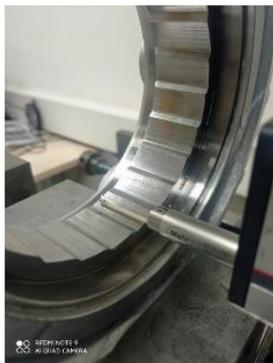
Fig. 5. A measurement of internal contoured surface
