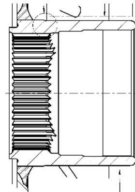
Fig. 1. A broach of the internal contoured surface
