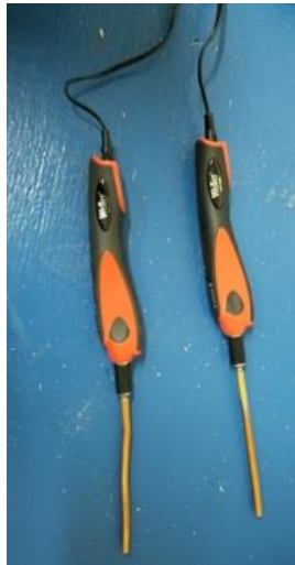
Fig.4. Weller Soldering Irons used as a heat source
