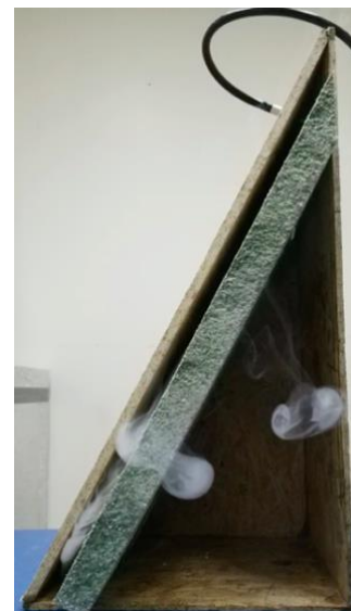
Fig.2. Introduction of smoke into the roof cavity
