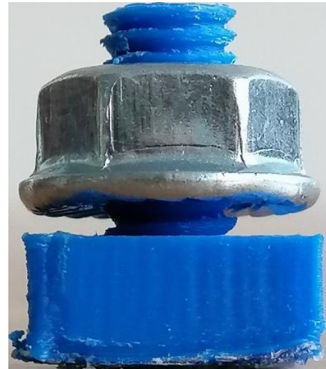
Fig. 12. Assessment of the printed piece by assembling it with a matching nut
