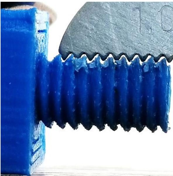
Fig. 11. Assessment of the printed piece with the feeler gauge
