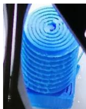
Fig. 7. Part filling for the Custom printing setup
