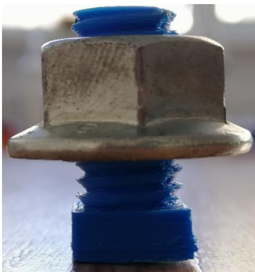
Fig. 3. Assessment of the printed piece by assembling it with a matching nut
