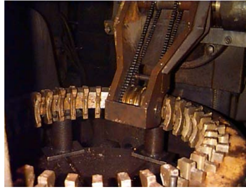
Figure 6. The helical worm – internal teeth worm wheel drive
