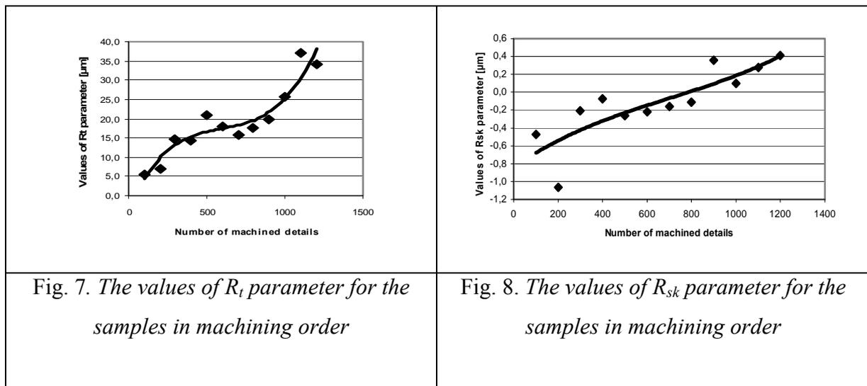
The measure of the asymmetry of the profile about the mean line is the parameter  $R_{sk}$ , called skeweness. Here (see Fig. 8) it has negative value up to 800th sample which means that the material is concentrated close to the peaks (the surface is like plateau with few valleys). For larger number of machined details  $R_{sk}$  rises to positive values, which means the material is concentrated lower (the valleys with few sharp peaks).
