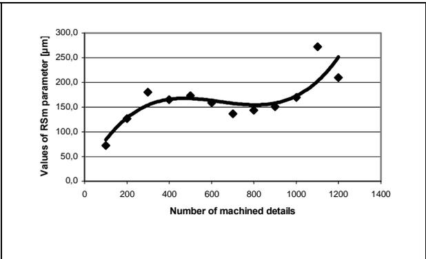
Fig. 10. The values of  $R_{Sm}$  parameter for the samples in machining order
