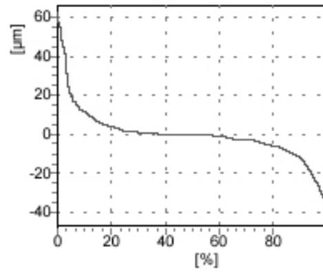
Fig. 11. The bearing ratio graphs for the samples No: a) 100, b) 700, c) 1100, d) 1200
