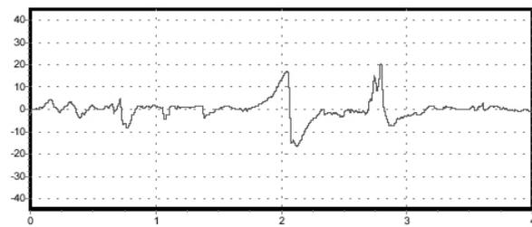
Fig. 12. Roughness profiles for successive samples (No 100, 200, 1000, 1100)
