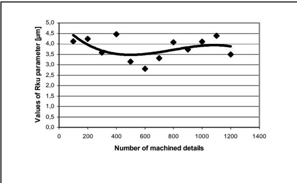
Fig. 9. The values of  $R_{ku}$  parameter for the samples in machining order
