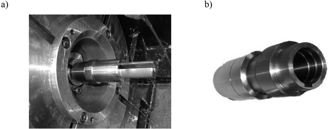
*Fig. 1. The pull broached detail: a) with tool leading pad, b) the detail with pull broached groove inside*
