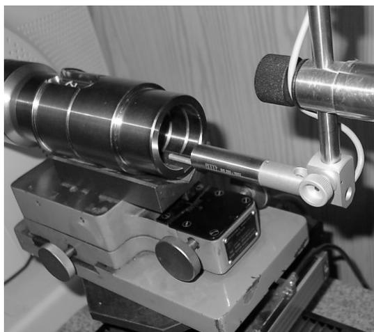
Fig. 3. *The measuring probe placed on the examined surface*
