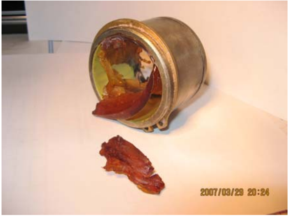
Figure 6. The failed PUR component
