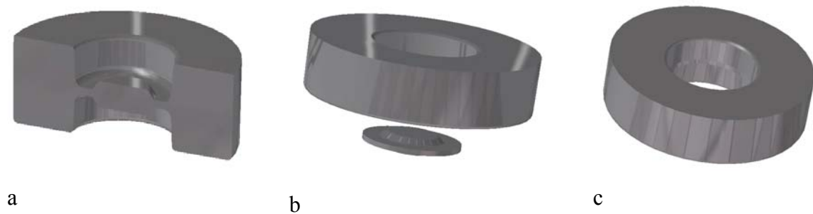
Fig.1 Model of die forging WHEEL a –shape of forged piece with wad and conical compensator, b –forged piece after punching of wad, c –shape of final forged piece
