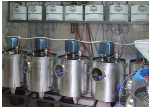
Fig. 1 The developed automatic fermentor line
