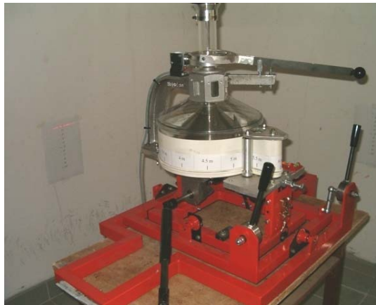
Figure 2: Examination of cone-belt dispenser
