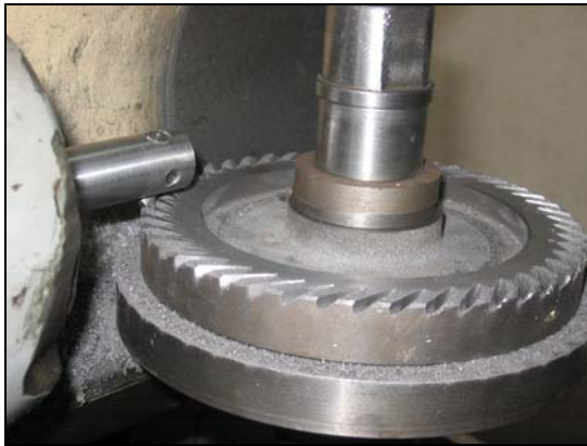
Fig. 8 Fly cutting lateral view
