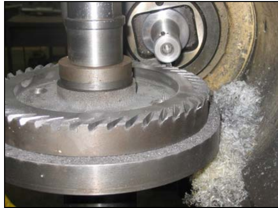
Fig.9 Fly cutting frontal view
