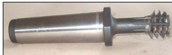
Fig.3. Spiroid hob for tangential advance
