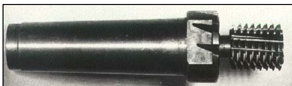
Fig.2. Spiroid hob for axial advance
