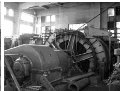
Fig.3 Extracting machine type 2T-3,5×1,7
