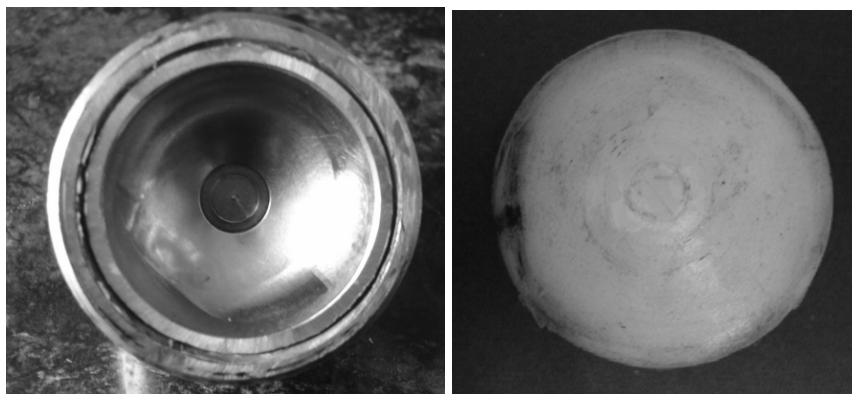
Fig. 3. The effect of wear on the prosthetic components: metallic endplate (left) and polymeric nucleus (right).
