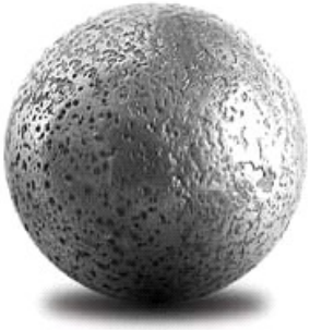
Fig.1. Electric pitting on a ball.
