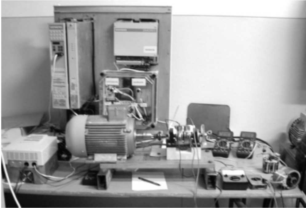
Photo 2. Test rig with two tested ball bearings.
