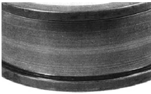
Fig.2. Ditches on the raceway.
