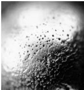
Fig.1. Electric pitting on a ball.
