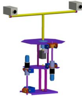
Fig.4 Designed mobile robot construction
