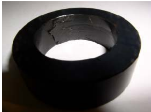
Fig.2. POM-H bearing with damaged running surface
