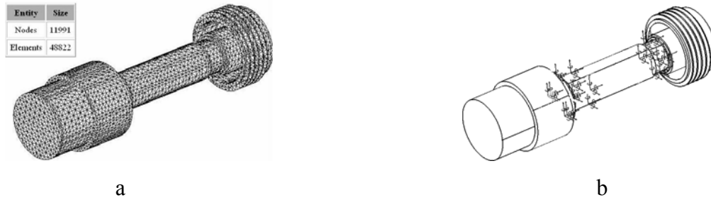
Fig.4. Spindle: a. discretization b. Model constraints
