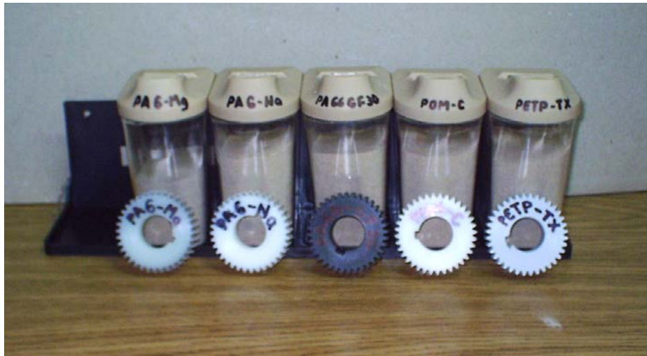
Fig.2. Tested polymer gears with the abrasive material
