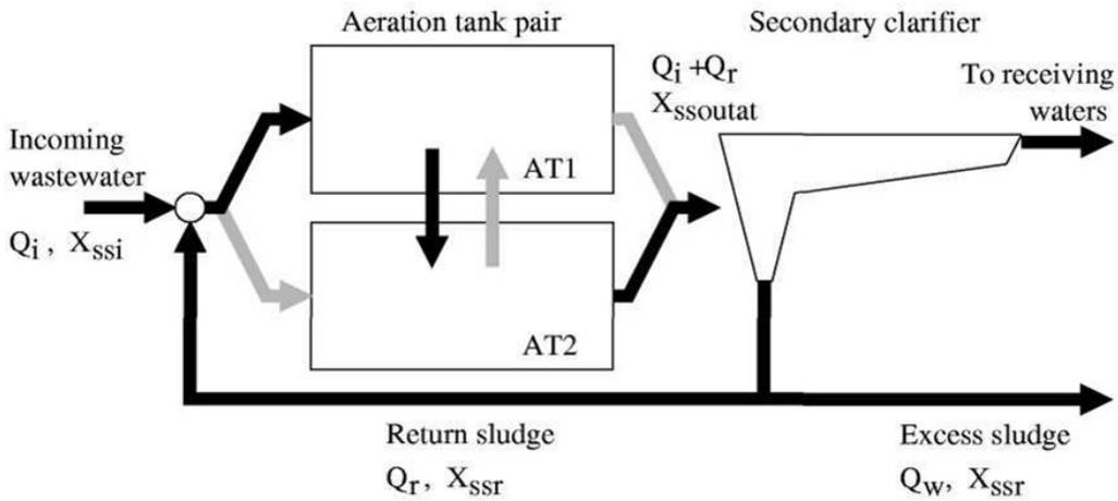
Figure 1. Flow path through aeration tank pair in an alternating WWTP
