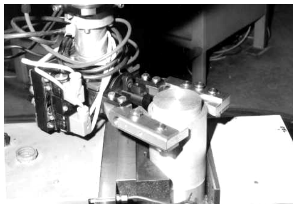
Fig. 4 Pneumatic sensory gripper during handling of cylindrical work piece
