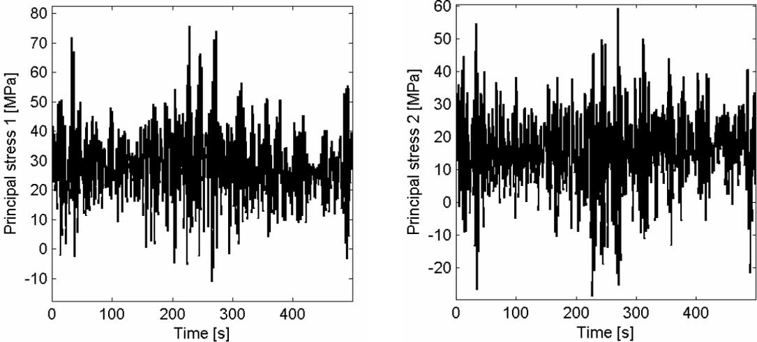
Fig. 7 Time behaviors of principal stresses  $\sigma_1(t)$  and  $\sigma_2(t)$  in damage critical
