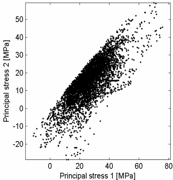
**Fig. 8** Non-proportionality of principal stresses in critical point
