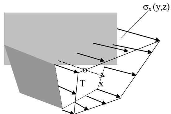
Fig.2 Distribution of the stress  $\sigma_x$  in a beam
