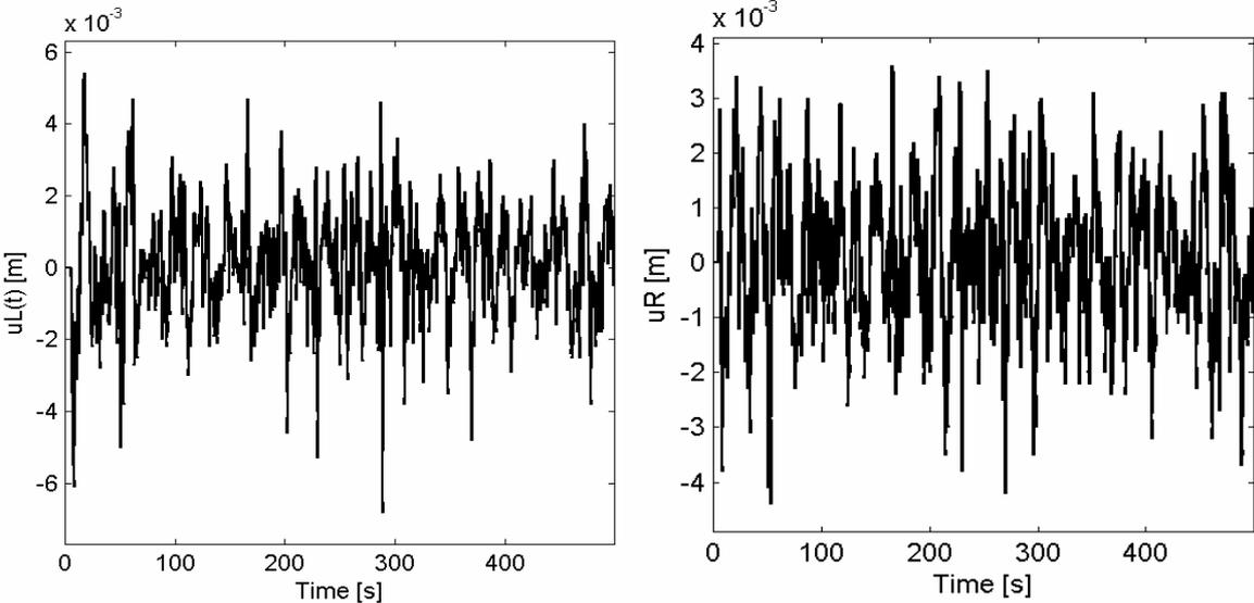
Fig. 6 Generated time behaviors of the vertical random axlebox displacements  $u_L(t)$  and  $u_R(t)$
