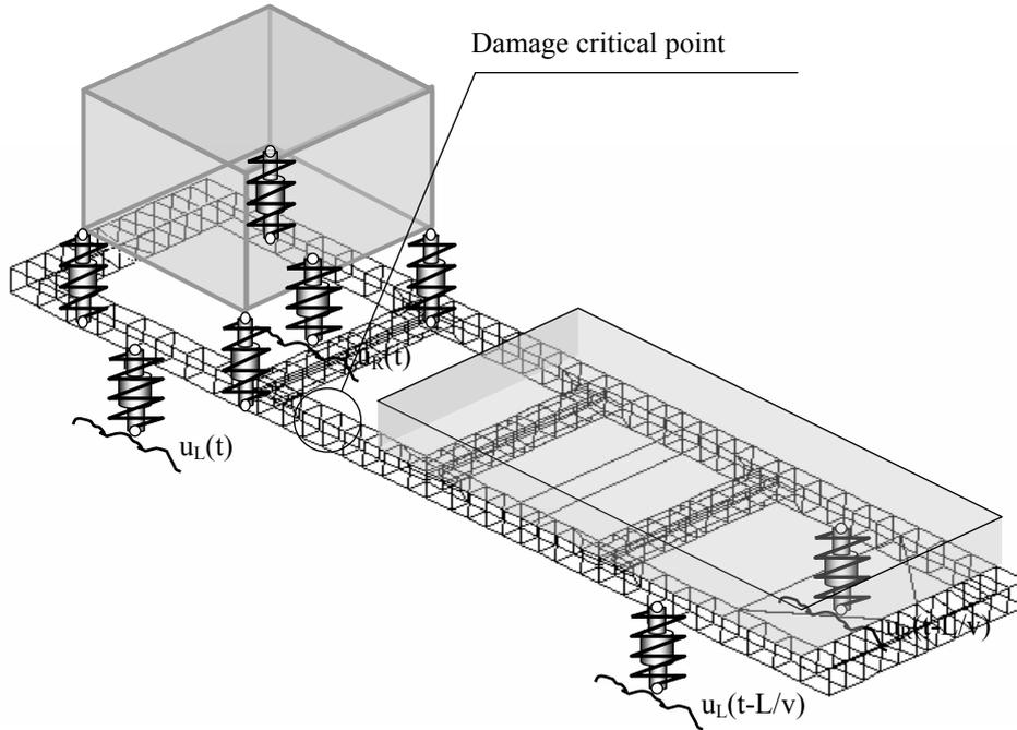
**Fig.4** Computational model of the machine DELTA with identification of the critical point subject to cumulative damage
