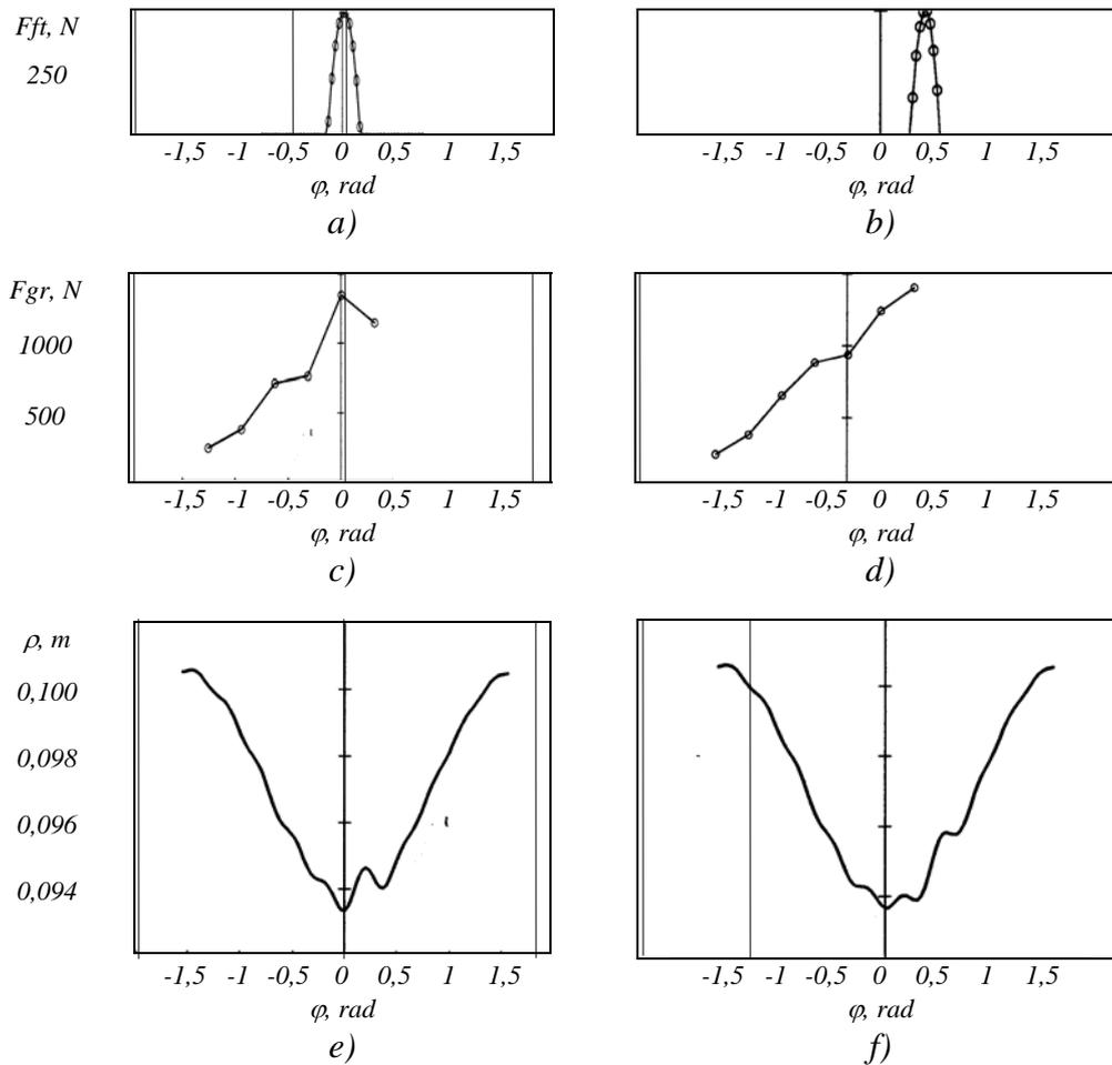
**Fig. 5.** Calculated values. a) and b) tangential tooth load, c) and d) radial generator load, e) and f) radius of curvature. a), c) and d) wave gear drive. b), d) and f) wave gear coupling.  $w_0/m = 1,1$ ,  $m = 1$  mm,  $r_0 = 97,1$  mm,  $h_e = 3,7$  mm,  $b_e = 80$  mm,  $M_2 = 600$  Nm
