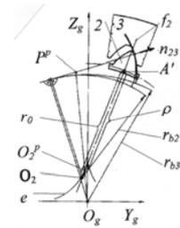
**Fig. 3.** Meshing of a tooth pair
