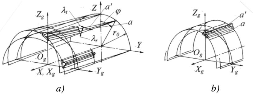
**Fig. 1.** Middle surface and teeth of a flexible gear a) Cup type flexible gear, b) Ring type flexible gear
