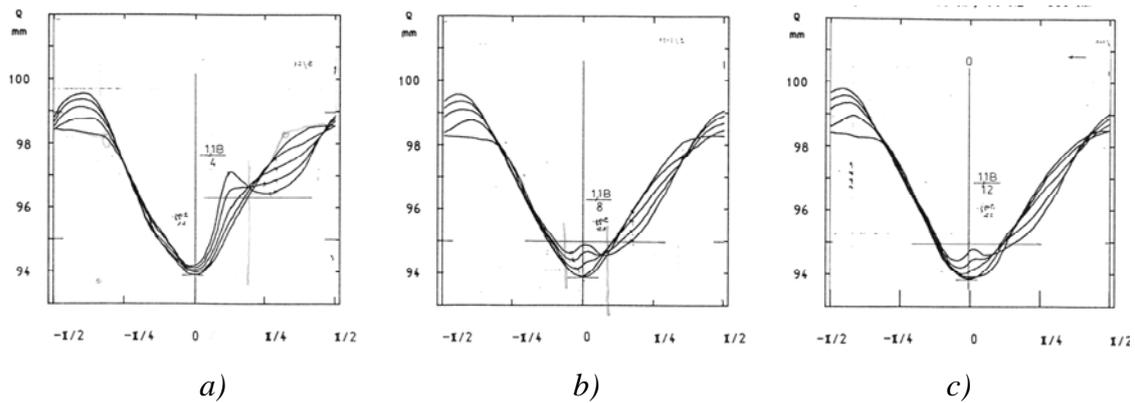
**Fig. 6.** Measured values of the radius of curvature. a) Flexible gear coupling. b) and c) Flexible gear drive,  $w_0/m = 1.1$ ,  $m = 1$  mm,  $r_0 = 97.1$  mm
