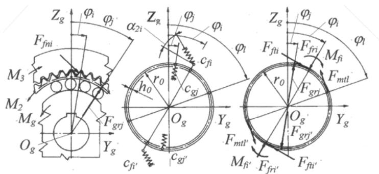
**Fig. 4.** Forces and moments acting on a flexible gear
