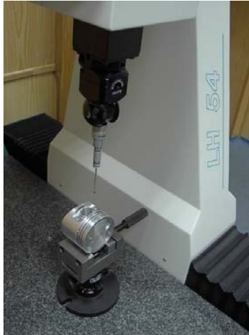
Fig.1 Piston measurement on WENZEL CMM
