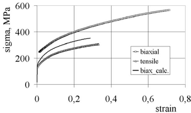
Fig. 4. Uniaxial tensile test and biaxial (bulge) test stress-strain curves of DDQ steel sheet
