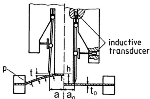
Fig. 1. Hydraulic bulge test apparatus
