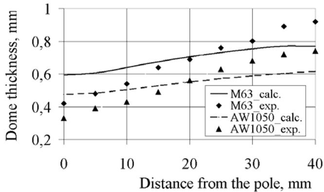
Fig. 3. Dependence of dome thickness on the distance from the dome apex of brass and aluminium sheet at the end of bulge test
