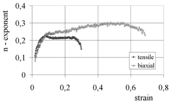
Fig. 5. Differential strain hardening exponent of uniaxial tensile test and biaxial (bulge test) of brass sheet
