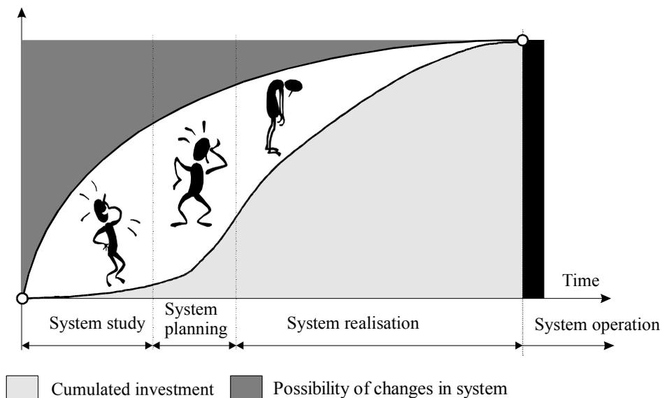
Fig.2. Possibilities of changes and costs of investment at different stages of project's realisation [1]
