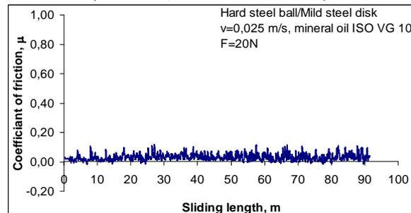
Fig. 12: Variation of the coefficient of friction of hard steel ball/mild steel disk (F=20 N, with lubrication)
