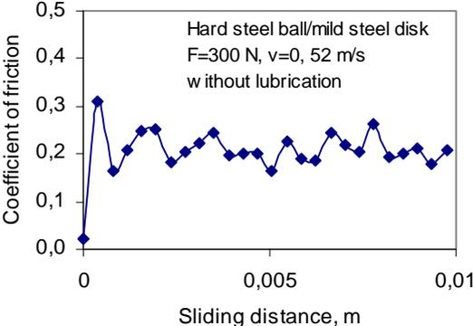
Fig. 2: Variation of the coefficient of friction of hard steel ball/mild steel disk at the beginning of experiments (F=300N)
