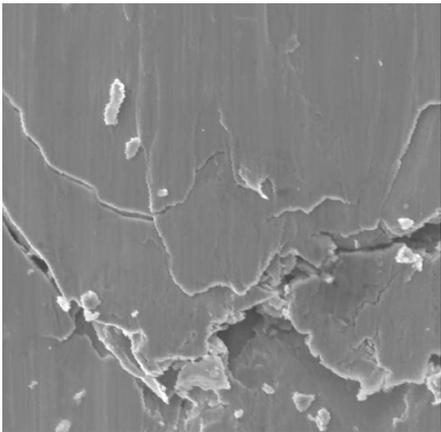
Fig. 3. Intensive plastic deformation in the middle of the wear track under load of 1200N.
