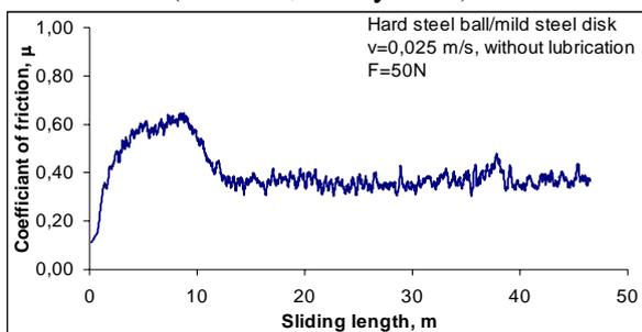
Fig. 9: Variation of the coefficient of friction of hard steel ball/mild steel disk (F=20 N, in dry case)
