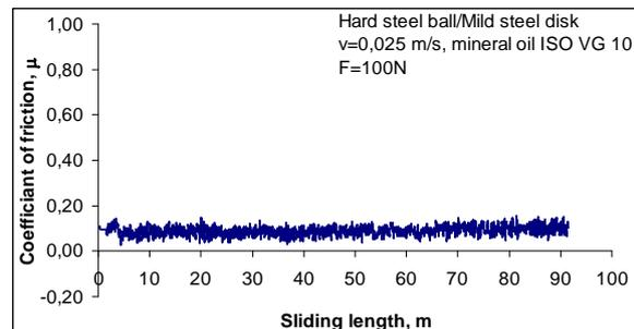
Fig. 10: Variation of the coefficient of friction of hard steel ball/mild steel disk (F=100 N, with lubrication)
