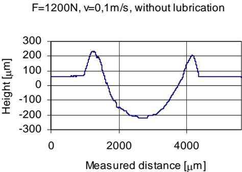
Fig. 5. Cross-section of wear track under load of 1200N.
