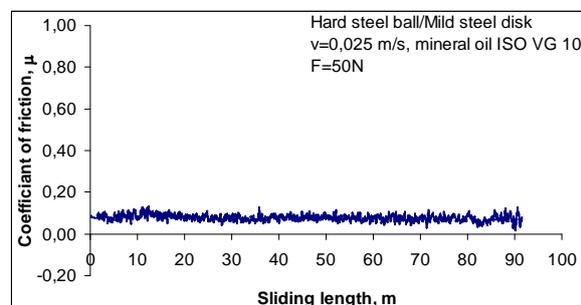
Fig. 11: Variation of the coefficient of friction of hard steel ball/mild steel disk (F=50 N, with lubrication)
