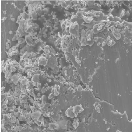
Fig. 4. Wear fragments in the middle of the wear track under load of 300 N.
