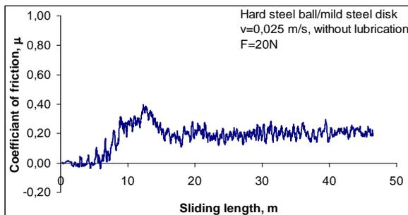
Fig. 8: Variation of the coefficient of friction of hard steel ball/mild steel disk (F=50 N, in dry case)
