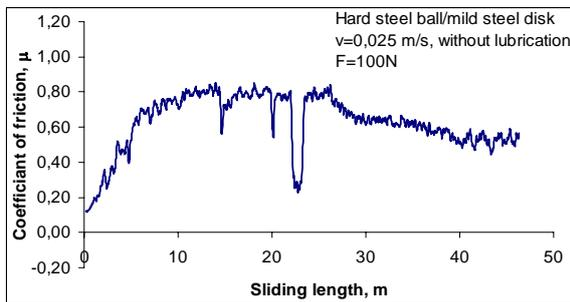
Fig. 7: Variation of the coefficient of friction of hard steel ball/mild steel disk (F=100 N, in dry case)
