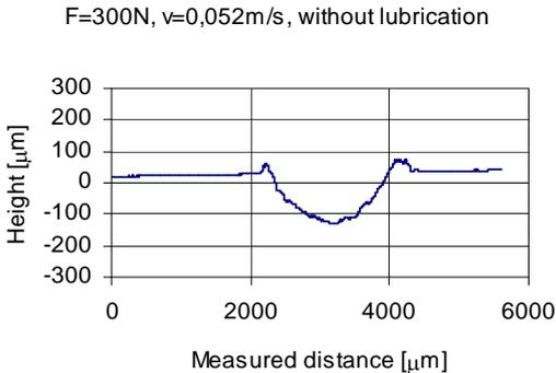
Fig. 6. Cross-section of wear track under load of 300 N.
