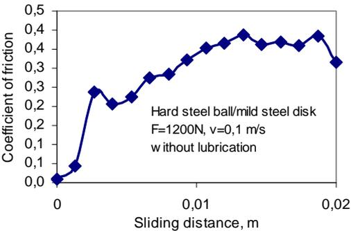
Fig. 1. Variation of the coefficient of friction of hard steel ball/mild steel disk at the beginning of experiments (F=1200N)
