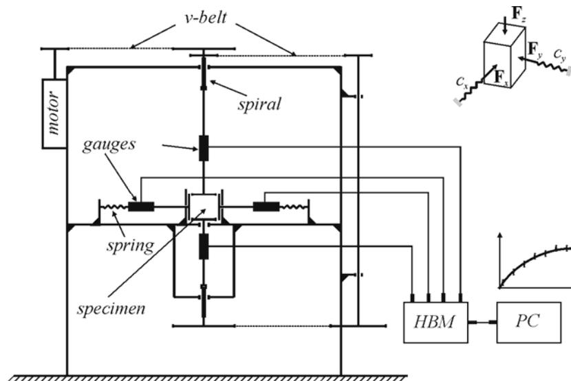
Fig. 1: Quasi-triaxial apparatus
