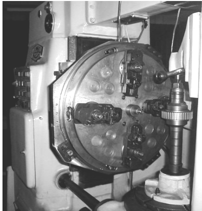
Fig.3 Multi-tool milling head
